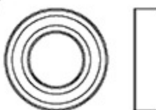
Bearing 軸承 (φ12xφ24x6mm) x 3
