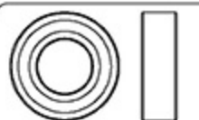
Bearing 軸承 (φ8xφ16x5mm) x 2
